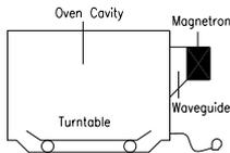
In a microwave oven, electricity is converted into microwaves by the **MAGNETRON**.
