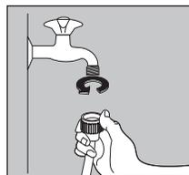
*When there is a inlet valve at the back of the machine, it must be connected to a cold water supply. If there are two inlet valve, one is connected to a cold water supply and the other is connected to a hot water supply. Follow the indication of the picture below to complete the connection.*
