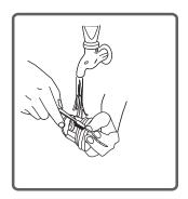
• After cleaning the filter, fit the filter cover and tighten it by rotating it in clockwise direction.
