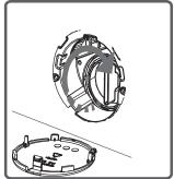
• While closing the pump cover, ensure that the parts on the inner side of the cover to match the holes on the front panel side.
