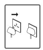
The mains cord of your washing machine is equipped with a specific earthed plug. This plug should always be inserted to a earthed socket of 10 amps.
